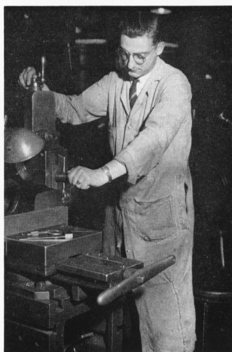
Felix Vitkauskas operates a Hendey power shaper. He is helping turn out tools for the production departments. Felix is a fife player in the Scovill Drum Corps.
