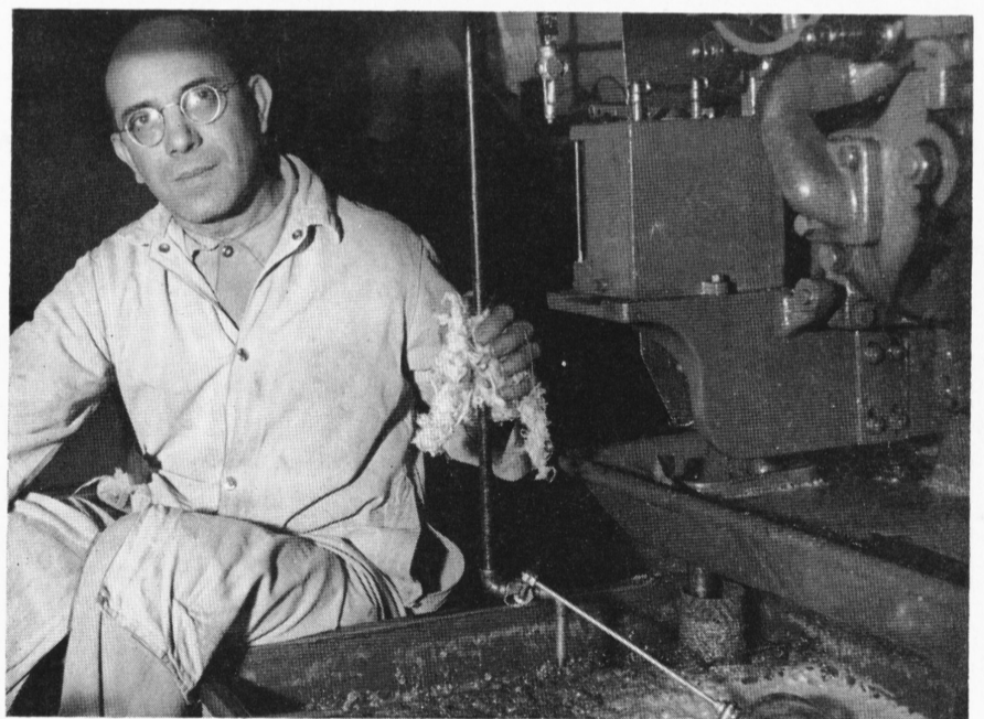
This gadget was adapted to serve as an automatic oil regulator on machines in the Automatic Screw Machine Department, by Charles Perrotti, a toolsetter in the Department, shown in the picture.
